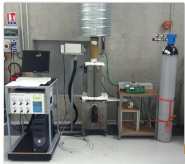
“Cracker “ : Tars-cracking test bench
