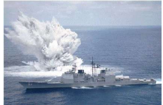
Ship subjected to underwater explosion
