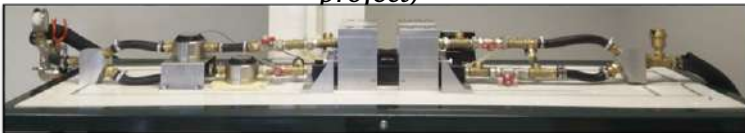
Test bench developed for the determination of Rth and Zth of wide gap components
