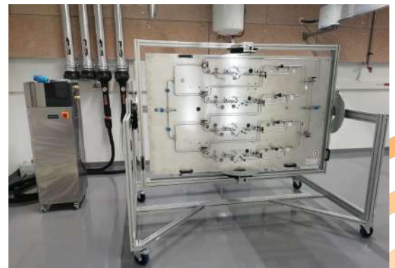
Test bench for the characterization of new micro-exchanger (SoCool project)
