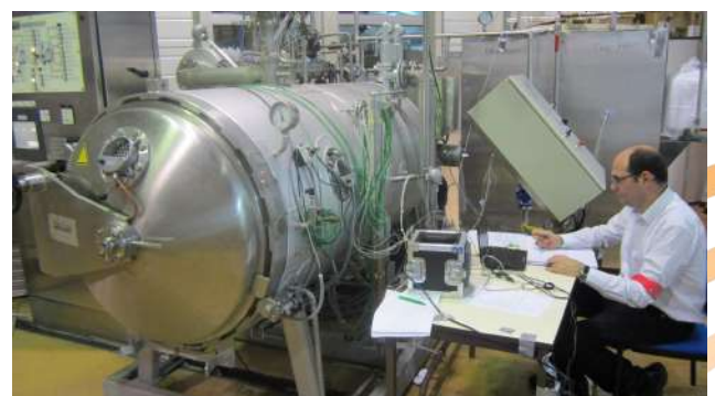
6kWh – 150kW PCM storage implemented on STERIFLOW sterilizer
